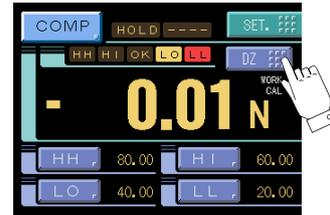
2) Press the [YES] button to perform the digital zero. Press the [NO] button to go back to the previous screen without executing digital zero. Press the [RESET] button to reset the digital zero.
